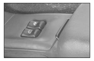
The switches on the center console control each of the power windows when the ignition is on. In addition, on four-door models, each rear passenger door has a control switch for its own window.
